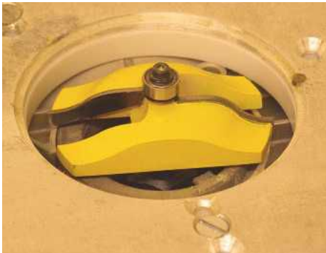
▲ Pic.10 Large-diameter cutters such as panel-raising types should be used only in a table-mounted router
